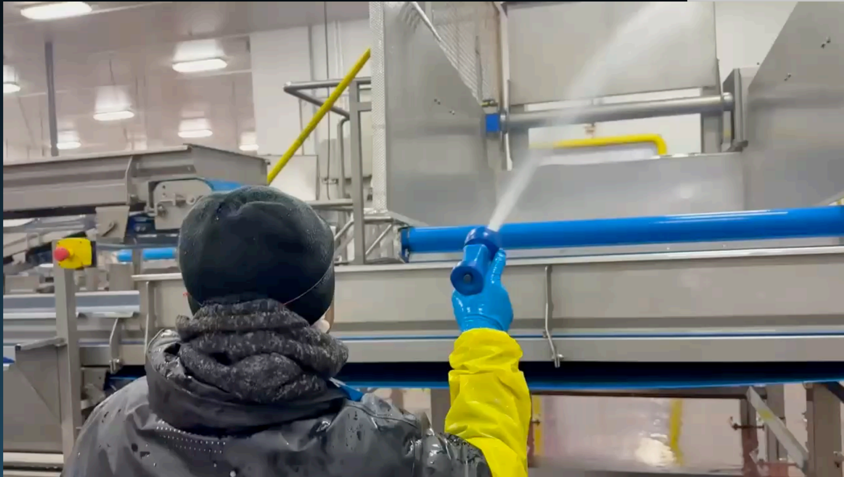
STEP 4: Post Rinse & Self Inspection
